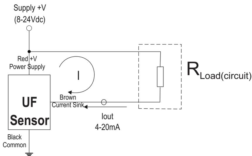
An ammeter (or suitably arranged multi-meter), placed in series at the lout point, will give an indication of the sensors current performance i.e. flow.
