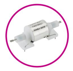
A complete RF screen around the coil assembly for a low loss transmission path, results in better carry current at elevated temperatures for this open frame series. An anti-corona sleeve is fitted around the reed switch for improved RF voltage isolation.
